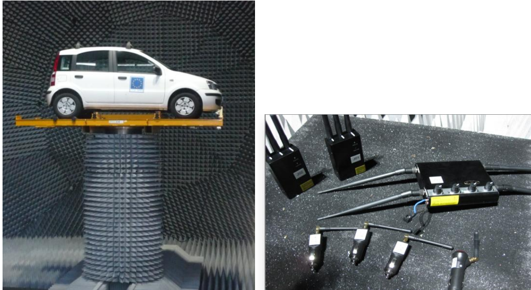
Figure 5 - Car being tested in anechoic chamber at IPSC, JRC (left). Sample of commercially available jammers tested (right).
